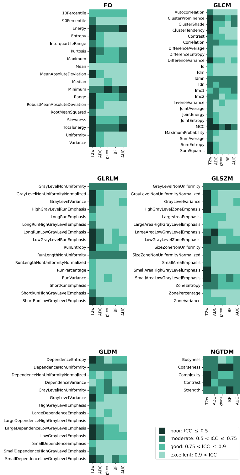
Figure 4. Result of the stability assessment of the radiomics feature values under contour variation within the six feature families for the T2-weighted (T2w) magnetic resonance image (MRI) and the 4 quantitative MRI maps, based on the interclass correlation coefficient (ICC), ICC(2,1) value. FO: first order, GLCM: gray level cooccurrence matrix, GLRLM: gray level run length matrix, GLSZM: gray level size zone matrix, GLDM: gray level dependence matrix, NGTDM: neighboring gray tone difference matrix, ADC: apparent diffusion coefficient, K trans : plasma transfer constant, BF: blood flow, AUC: area under the curve.
