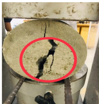
Figure 4. Bridging effect of fiber.
