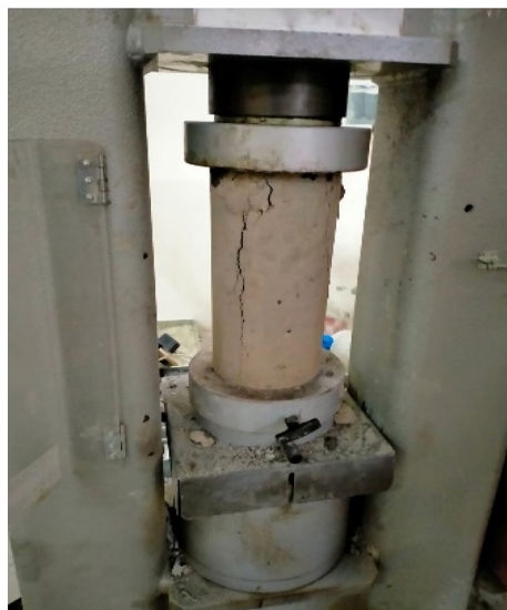
Figure 3. Compressive strength test.
