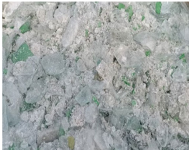
Figure 7. Waste glass after washing and drying.
