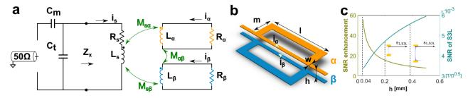
**Figure 2.** (a) Circuit model of the saddle coil, inductively coupled to the S3L insert for SNR enhancement. (b) Dimensional parameters of the S3L geometry. (c) Calculated SNR enhancement and absolute SNR versus stripline spacing h based on the circuit model, and profiles of the  $B_1$ -field distribution between two striplines (yellow blocks) respectively with h = 200, 390 µm.
