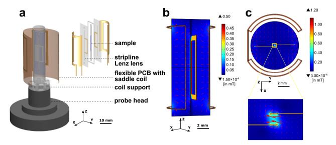
**Figure 1.** Configuration of a stripline Lenz lens chip on an NMR probe-head, and its magnetic field distribution. (a) Illustration of the coil system with a saddle coil and an S3L chip mounted on the probe head. Exploded view of the coils, with the sample region shaded blue. (b)  $B_1$ -field distribution on the xz-plane via a color map, and an arrow surface plot. (c)  $B_1$ -field distribution on the xy-plane, and a zoom-in view around the stripline.
