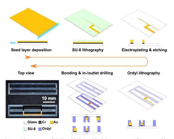
**Figure 7.** Fabrication process of S3L chip with both 3D model and 2D cross-section, as well as a top view of the fabricated S3L chip alongside with a dummy chip.
