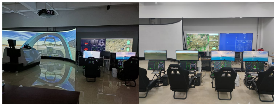
Figure 10. The experimental setup utilized in this study included a full-scale cockpit of a combat aircraft and a three-channel simulation testing platform.
