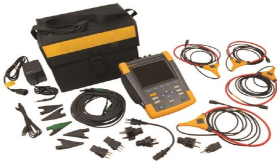
Figure 1. Power quality analyzer device 11 .
