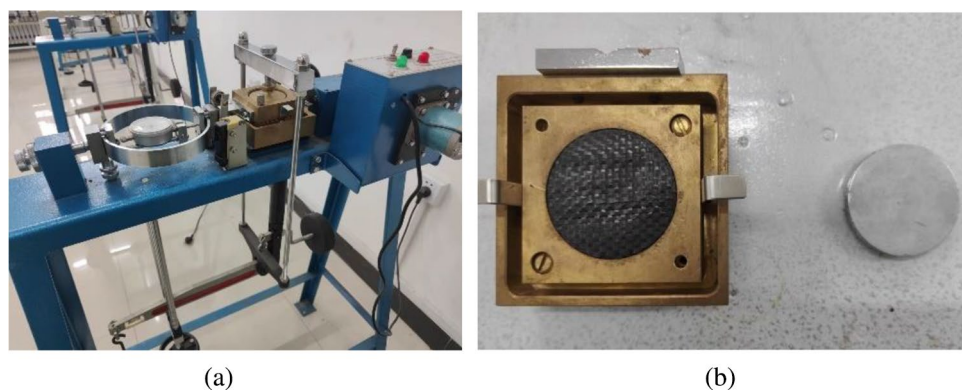
Figure 6. Test equipment and shear interface: (a) ZJ-2 strain-controlled straight shear equipment, (b) geosynthetics and metal plate interface.
