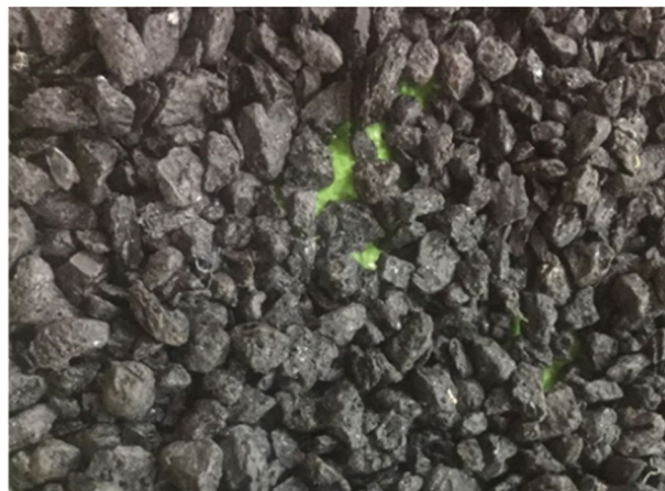
Figure 2. E-waste coarse aggregates obtained from electronic waste.
