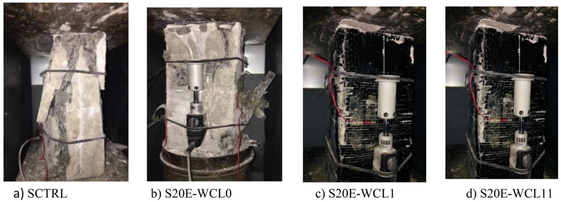
Figure 15. Patterns of failure in square samples.
