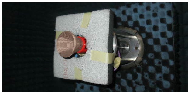
Figure 4. 3D-printed antenna measurement in anechoic chamber.
