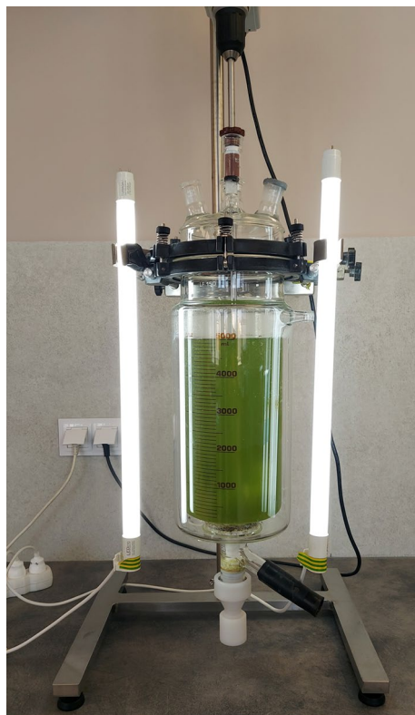
Figure 1. Installation with a photobioreactor used for the experiment.
