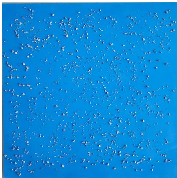
Figure 2. Experimental gravel distribution on an 1 m × 1 m blue PVC plastic plate.
