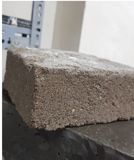
Figure 5. Block stabilised at 3% AAS.
