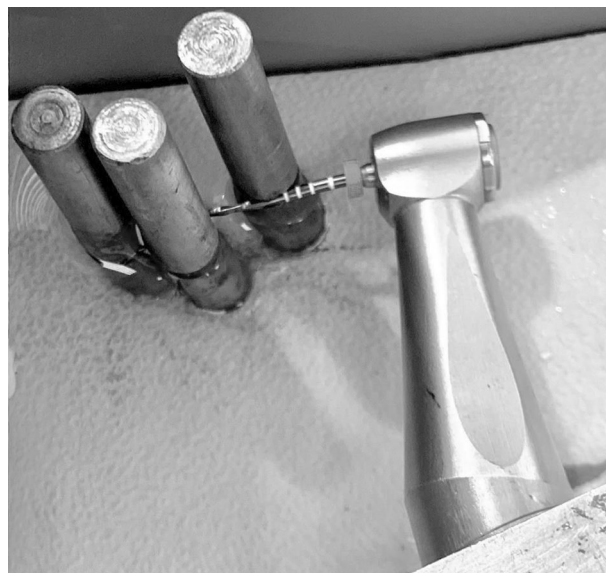
Figure 2. The equipment employed for conducting the cyclic fatigue test.
