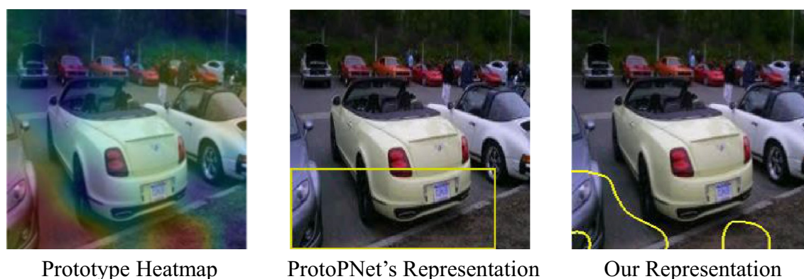
Figure 3. Examples of complex prototype heatmaps and the failure of a rectangular prototype representation. While the actual heatmap (left) points to irrelevant background regions, the rectangular representation (center) misleadingly includes foreground regions. Our solution (right) properly represents the actual heatmap.
