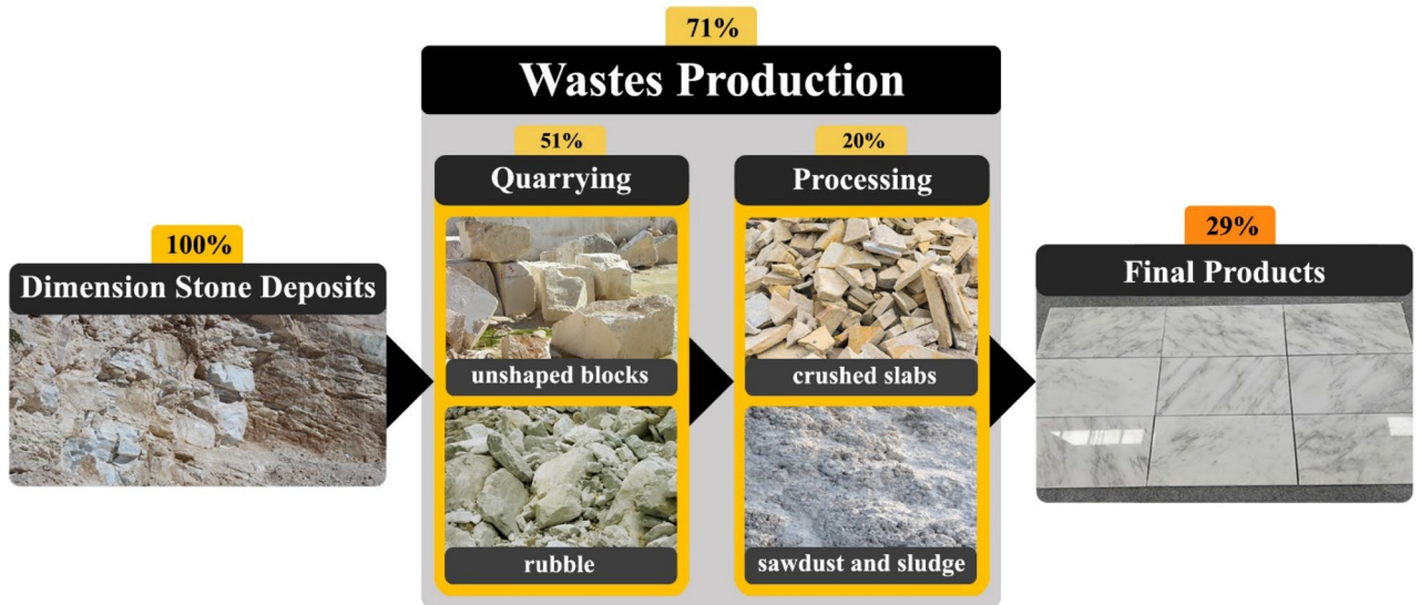
Figure 2. Products and wastes in different stages of the dimension stones production cycle.
