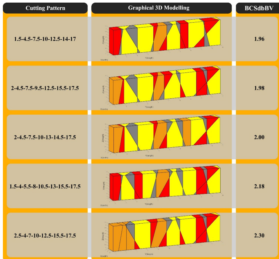
Figure 13. The first five cases of the best cutting patterns proposed by the optimization algorithm for "Model 1".
