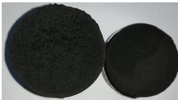
**Figure 5.** Internal moisture of coal sample after the experiment.
