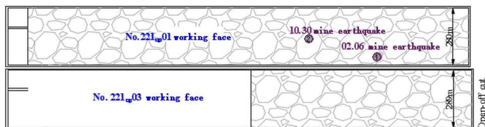
Figure 1. The layout of 221 Upper 01 and 221 Upper 03 working faces in Shilawusu.
