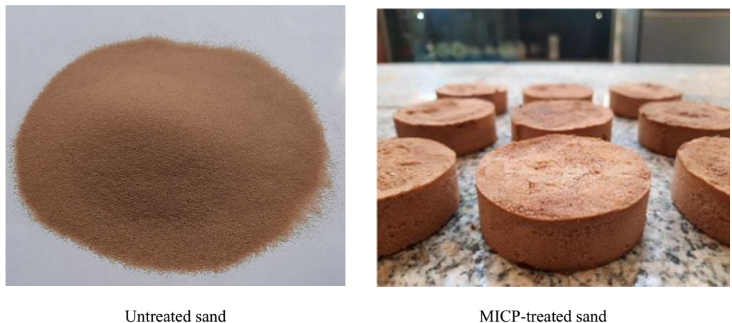
Figure 3. Sandy soil specimens: untreated vs. MICP-treated.
