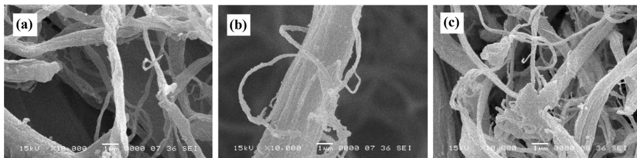
Figure 3. SEM images of: (a) untreated CMF, (b) CMF-TEOS, and (c) CMF- HDTMS.
