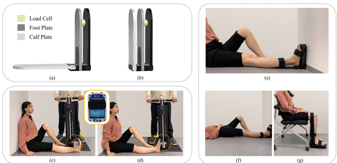
Figure 4. (a) 90° formation and (b) folded formations of the designed portable dynamometer; subject position for (c) ankle dorsiflexion strength measurement and (d) ankle plantar flexion strength measurement using the HHD; (e) long sitting, (f) supine, and (g) seated positions for ankle strength measurement using a portable dynamometer. (Figure of HHD is presented within (c) and (d)).
