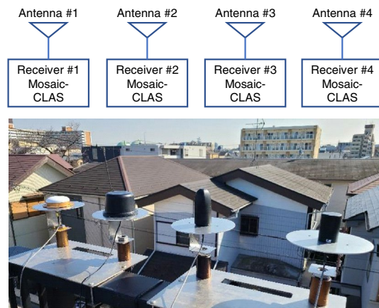
Figure 3. Experimental configuration and photographs of the antenna performance evaluation in a static test in an open-sky environment. GNSS observations are acquired simultaneously from four antennas for 24 hours. Each antenna is equipped with a 150-mm-diameter ground plane.
