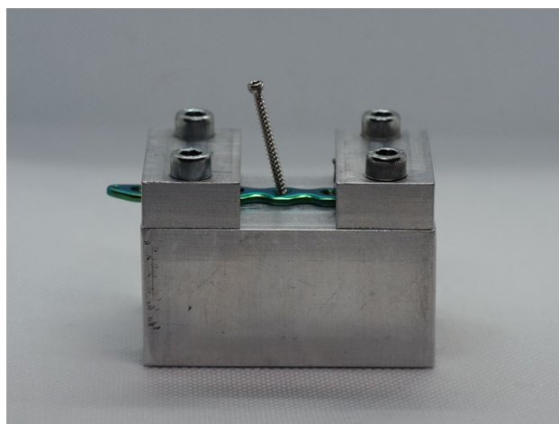
Figure 1. Pre-formed angulated block and 4.0 ChLP plate.
