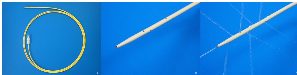
Figure 1. A dedicated 7-Fr catheter for lavage and aspiration. (A) The tip of the catheter was highly tapered to reduce the gap with the guidewire, and eight side holes were created within 25 mm of the tip. (B) This structure achieves excellent bile aspiration and high-flow washing with saline. (C) photograph of spraying saline.
