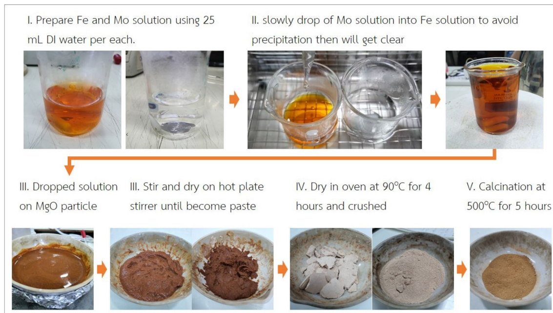
Figure 1. Preparation of FeMo/MgO by impregnation method.
