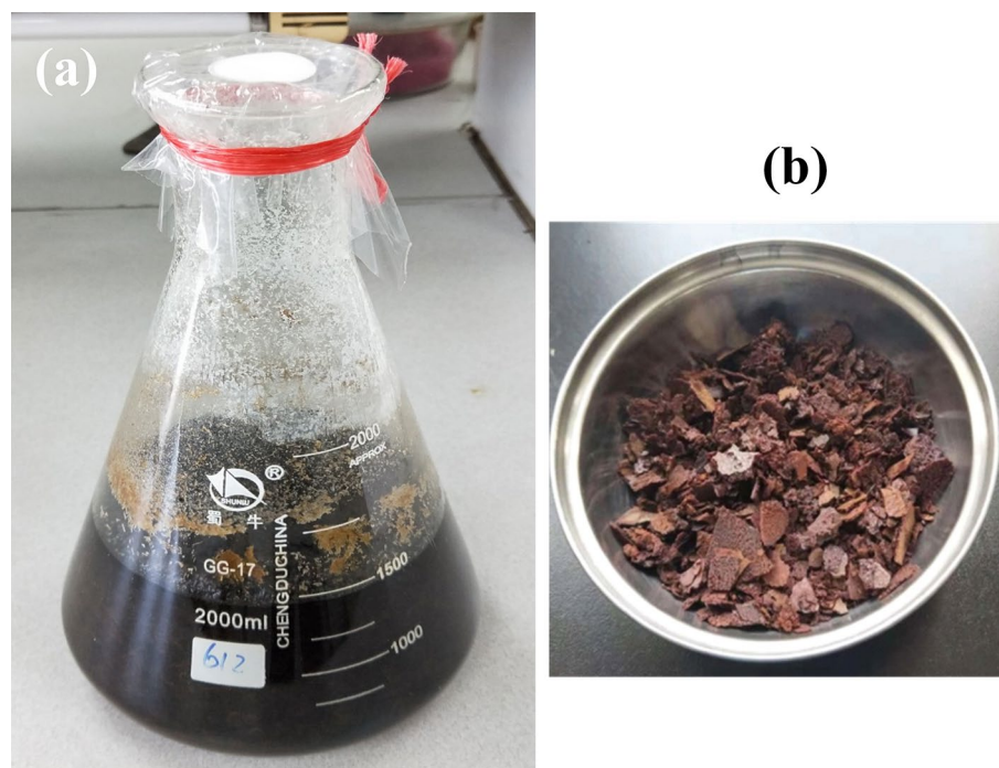
Figure 4. The photos of the saccharized sugarcane pith and sugar. (a) A photo of hydrolyzed sugarcane pith in phosphoric acid solution. (b) A photo of the sugar hydrolyzed from sugarcane pith. The remaining phosphoric acid in the dried sugar will play the role of activation reagent in activation reaction.
