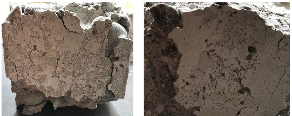
Figure 5. Pictures of used concrete after freezing and thawing cycle with resulting mass loss.
