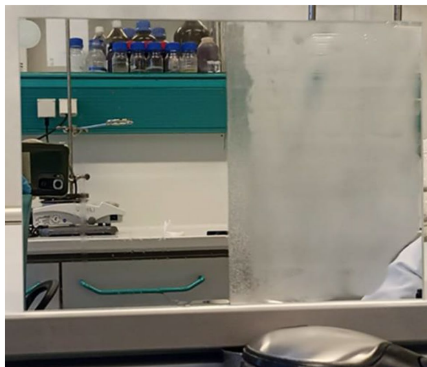
Figure 13. Photograph of uncoated (right side) and coated with derivative S4 (left side) mirror under the antifogging test.
