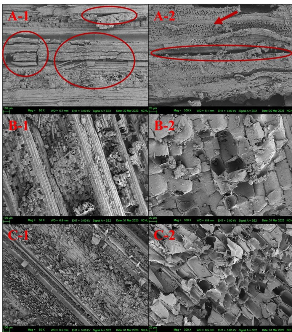
**Figure 2.** SEM images of (A) BS, (B) MB and (C) TB (Code 1 and 2 are associated with  $\times 50$  and  $\times 300$  magnification, respectively).
