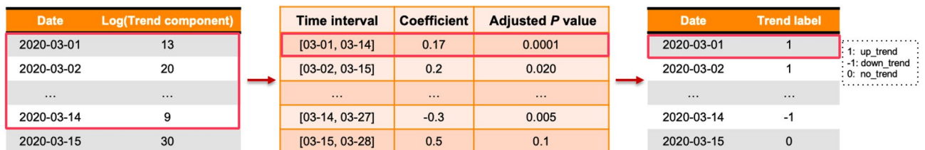
Figure 2. Illustration of fitting the log-linear regression model and identifying the corresponding trend of each date. Surveillance and digital traces data is fitted within a successive 14-days time interval (sliding window). For each sliding window, the statistically significant coefficient and adjusted P values are calculated, e.g. An “up-trend” (1) is given for the sliding window as the coefficient \beta is larger than 0 and the adjusted P value is less than 0.05 threshold.
