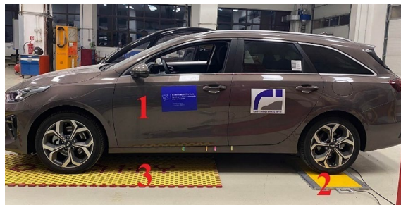
Figure 1. Principle of determining the axle load via portable weighing system: Tenzováhy PW-10.
