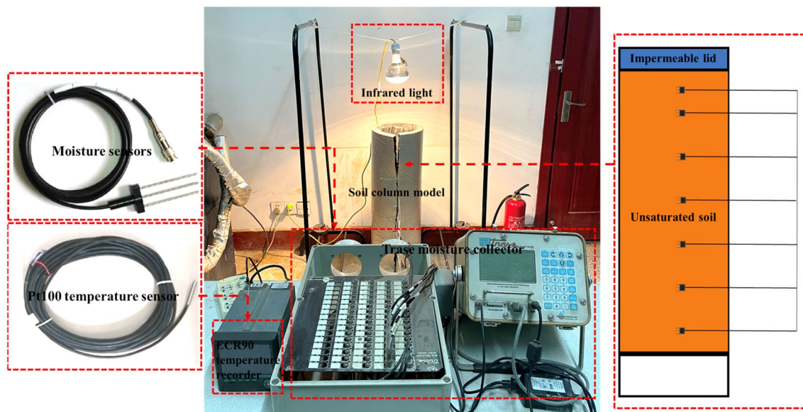
Figure 2. Moisture migration test devices.
