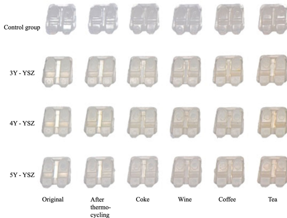
Figure 3. Changes in the appearance of the experimental and control bracket groups over time.
