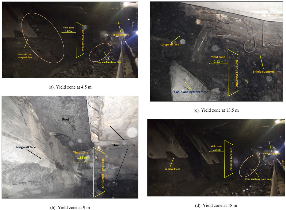
Figure 11. Yield zone of the longwall face observed in the study mine.
