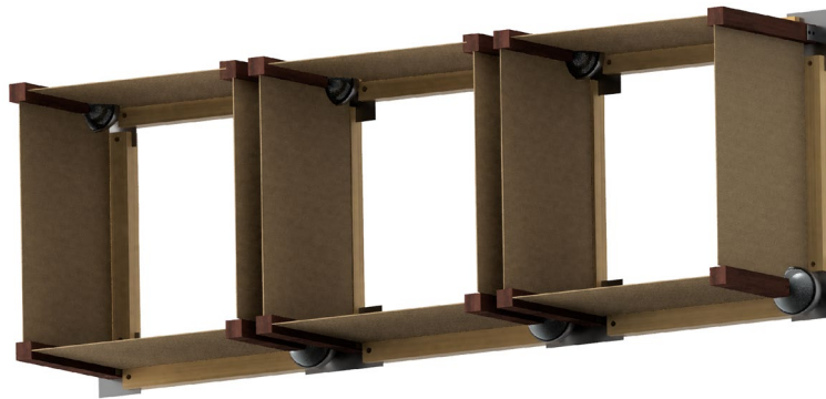
Figure 5. A Graphical computational model of the 3-module proposed adaptive façade, each consisting of 2 fixed and 2 spherical joints. Source by the authors.
