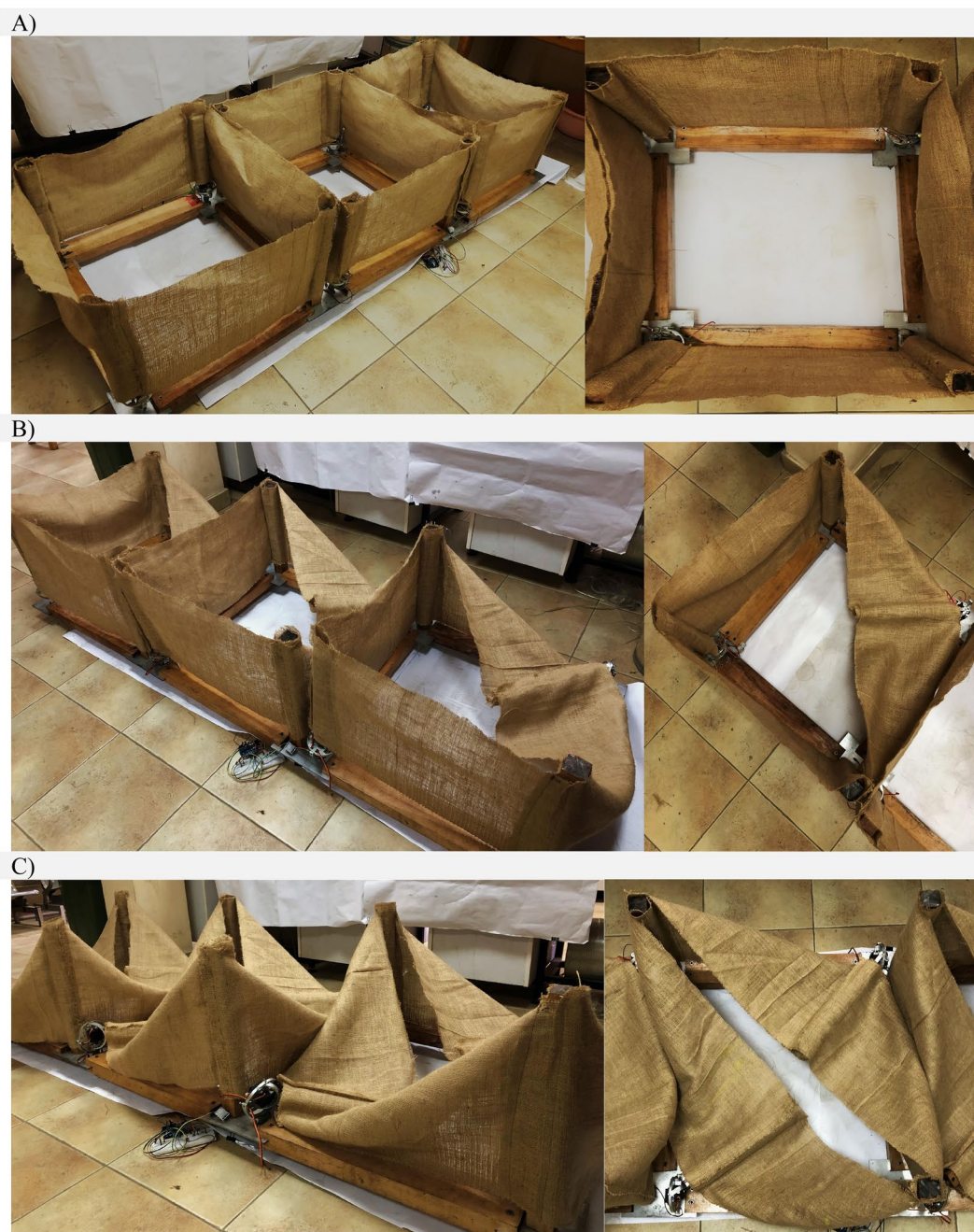
Figure 10. Fabricated prototype of the proposed adaptive modules and experiments. Each expected module state is presented across a single module, and the fabricated 3- module cluster. (A) The module is in fully open state when no shading is needed. (B) Intermediate state when partial shading is needed. (C) Almost closed state when maximum low-level sunrays are found.
