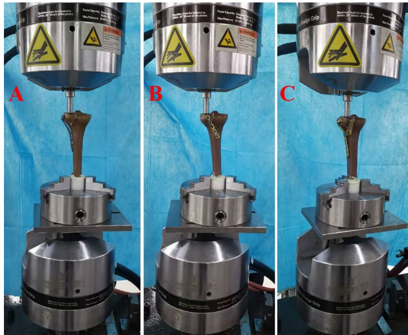
Figure 5. Positioning of three different tibial models within the biomechanical machine. (A) Fixation of the lateral locking plate in the PLTP fracture. (B) Fixation of the posterior buttress plate in the PLTP fracture. (C) Fixation of the novel plate in the PLTP fracture. PLTP posterolateral tibial plateau.
