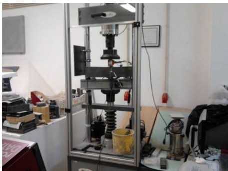
Figure 9. Fracture energy determination test.
