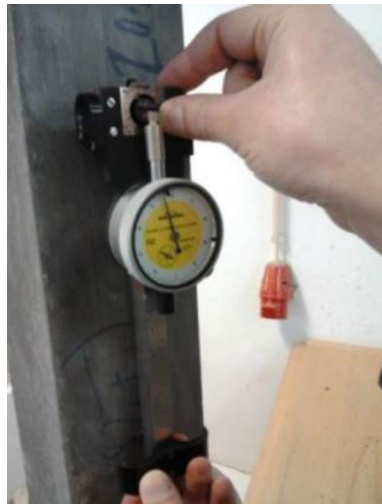
Figure 7. Test to determine the modulus of elasticity in compression.
