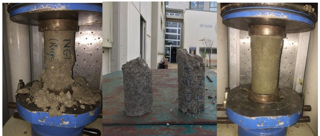
Figure 9. The 7 Day Compressive Strength Test for RM1, RM2, and RM3.
