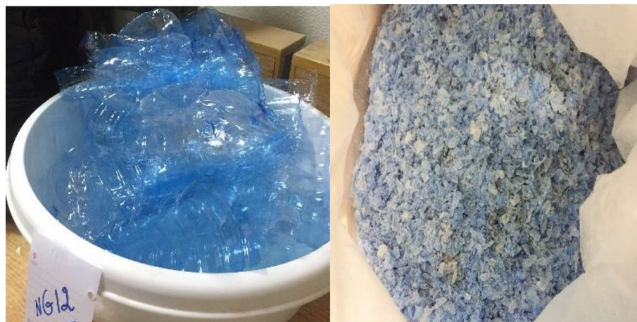
Figure 1. Plastic Bottles Before Shredding and after Shredding.
