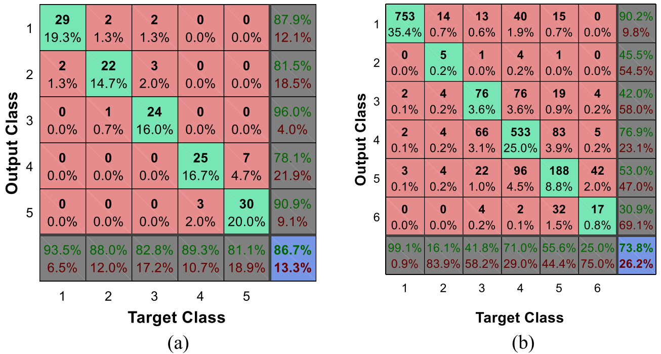
Figure 10. Confusion matrix of the combination of ECOC and decision tree for emotion recognition in the dataset (a) Berlin, (b) ShEMO, after 10 folds of cross-validation.
