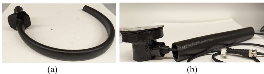
Figure 6. Encapsulated assembly for (a) vertical exit sensor, and (b) side exit sensor.
