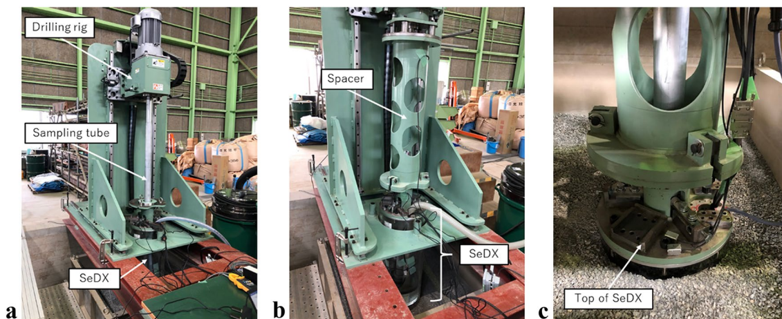
Figure 10. Model test: (a) set-up (corresponding to Fig. 5a); (b) before SeDX excavated the ground (corresponding to Fig. 5d); and (c) after SeDX excavated the ground (corresponding to Fig. 5e).
