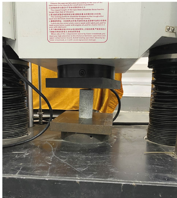
Figure 2. The uniaxial compression test process for rocks.
