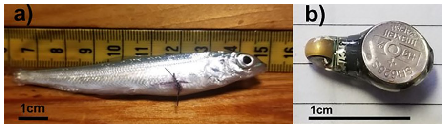
Figure 2. Acoustic-tagged juvenile fish. Juvenile cisco ( Coregonus artedii ) re-introduced from extirpation in Keuka Lake, New York, USA. (a) Juvenile cisco with a surgically implanted acoustic transmitter. (b) A small (0.6 g) acoustic telemetry transmitter used for age-0 fish in this study. Photographs by M. Chalupnicki, USGS.
