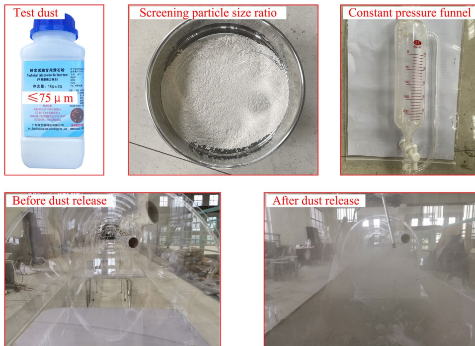
Figure 5. Experimental dust disposal.
