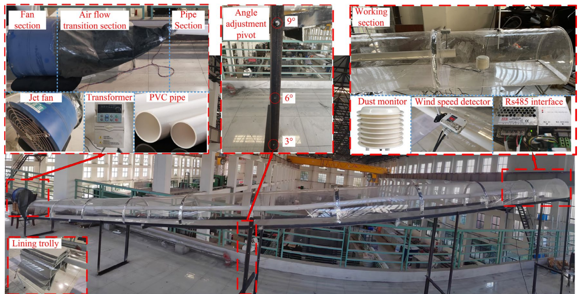
Figure 4. Tunnel model physical picture.
