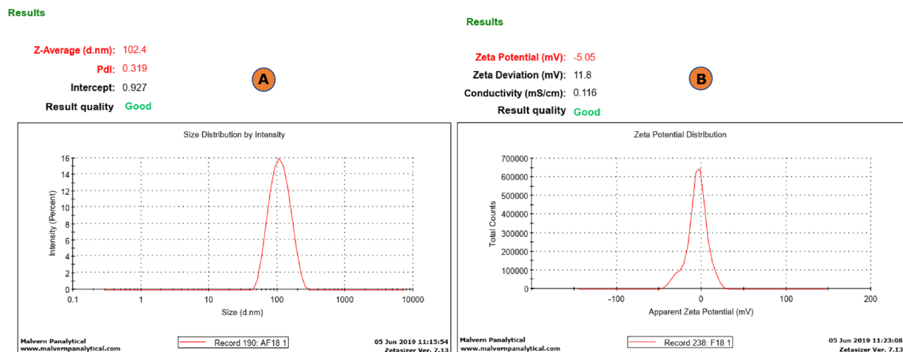
Figure 2. (A) Depicting vesicles size distribution and PDI; (B) Zeta potential of deformable-emulsomes.
