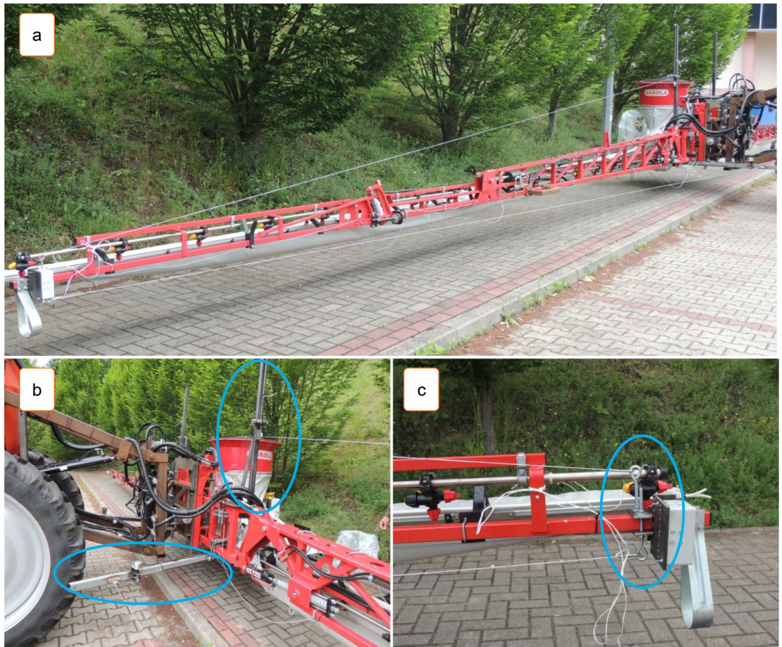
Figure 2. System for measuring the sprayer boom’s displacement from a state of equilibrium: (a) general view; (b) support arms with reel spools and cable tension springs; (c) loop screws for attaching measuring cables.
