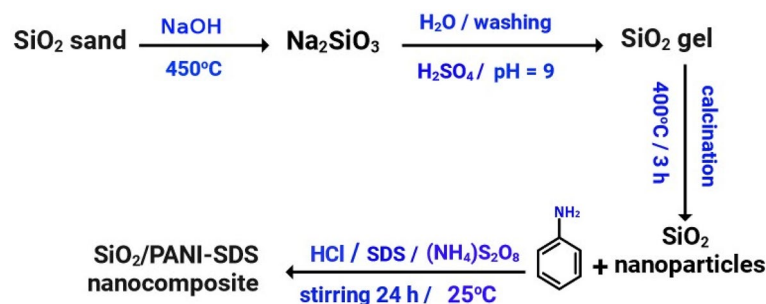
Figure 2. Synthesis of Silica nanoparticles and \text{SiO}_2 /PANI-SDS nanocomposite.
