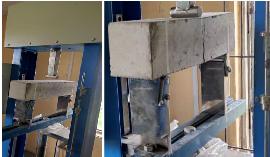
Figure 3. Beam sample undergoing flexural strength test.
