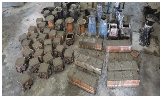
Figure 2. Freshly cast concrete cubes, cylinders and beams.
