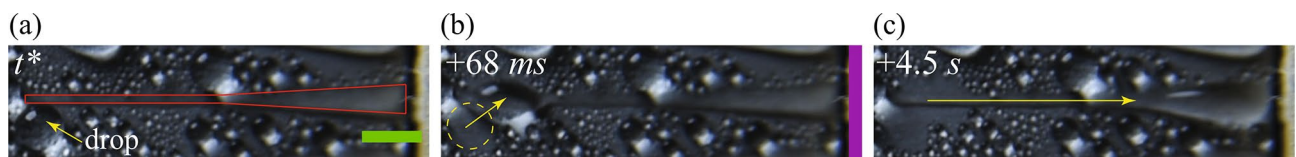
Figure 8. Illustration of liquid transport from the thin SHL rectangular track to the wider end of the wedge in the pattern P4. The red solid line represents the transition line between the SHB and SHL areas. The yellow arrow line represents the direction of liquid transport. The violet-coloured shaded region represents the side end of the wicking reservoir. The scale bar is 3 mm.
