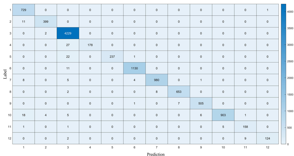
Figure 8. Confusion matrix. 1: Mussel boat; 2: sailboat; 3: passengers; 4: tugboat; 5: Dredger; 6: natural ambient noise; 7: motorboat; 8: RORO; 9: fishboat; 10: ocean liner; 11: trawler; 12: pilot ship.
