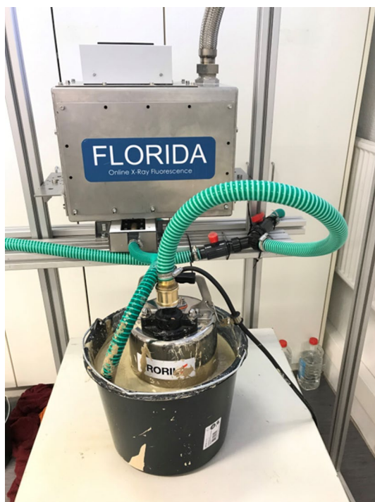
Figure 4. Setup built for the analysis of phosphate slurry in horizontal flow.
